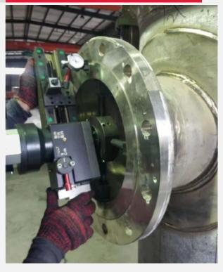
3 Machining the flange facing & grooves
